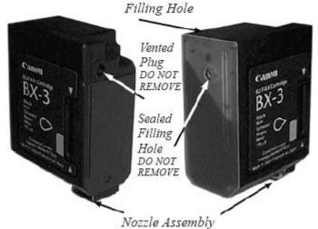
Use the plug provided or a piece of strong tape to seal the filing hole.
